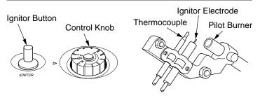
Figure 22 - Control Knob In The OFF Position
